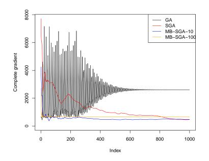
The original gradient ascent algorithm oscillates drastically. The stochastic versions seem to be converging away from 0 as well. Thus, the value of t is critical to implementing the (stochastic) gradient ascent algorithms in a stable way.
