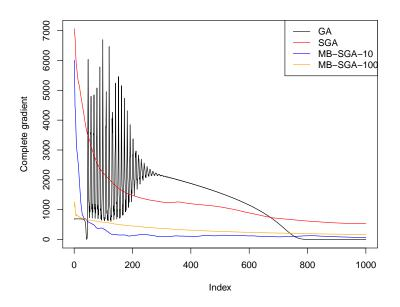
Note here that although the algorithm begins oscillate, due to decreasing step-sizes, the algorithm escapes out of local oscillations.
