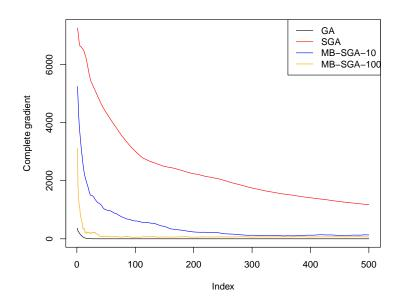
We see that the original stochastic gradient ascent algorithm is slow to converge although it is the cheapest. The mini-batches are far more stable.
